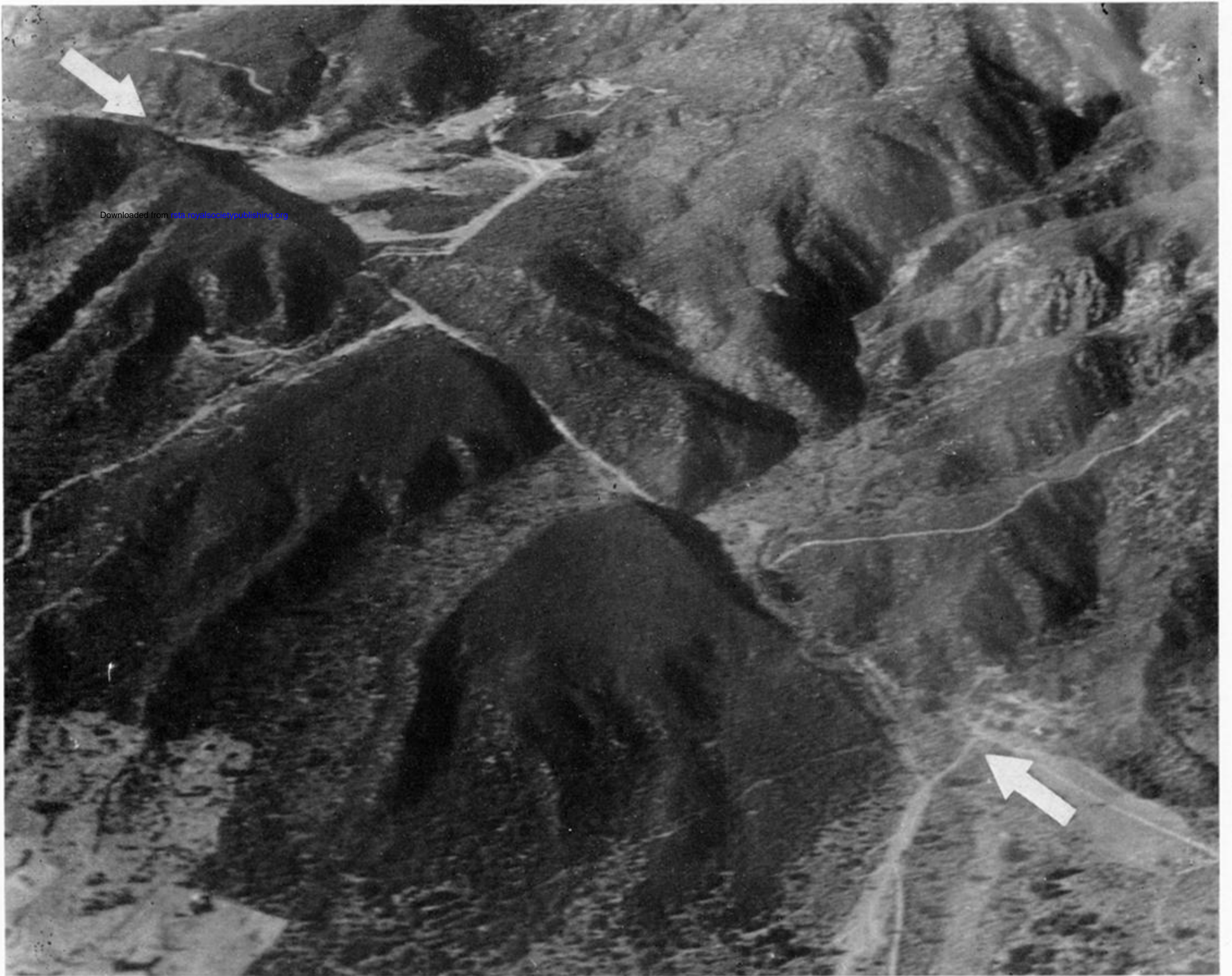
FIGURE 4. Dextral offsets of canyons along San Jacinto fault near Anza, California. Distance along fault between arrowheads is 1.9 km.
